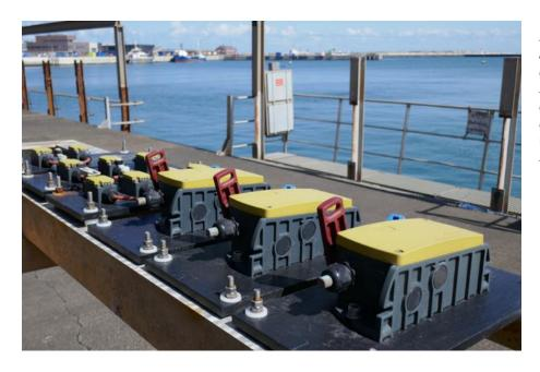
Interim checks after seven months of outdoor exposure on the island of Helgoland: the emergency pullwire switches are still fully functional
