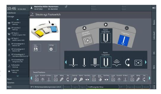
Fig. 4: Wireless enables: via a central user interface (foot switch and monitor/ keyboard), multiple medical devices can be selected and operated
